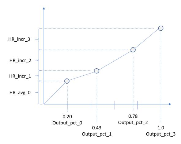
Fuel curves are stored in the Egret generator dictionary as p\_fuel. Values in the fuel curve are in MW (rather than output percent) and MMBTU/hr (rather than BTU/kWh). Fuel costs are calculated by interpolating the fuel curve for the current output rate, then multiplying by the fuel\_cost.
