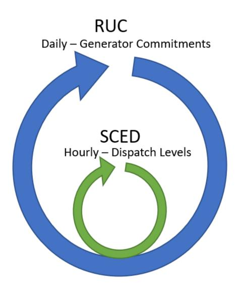
Prescient simulates the operation of a power generation network throughout a study horizon, finding the set of opera-
